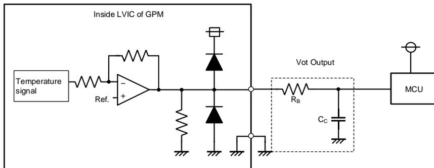
**Figure 5. Internal Block Diagram and Interface Circuit of V<sub>OT</sub>**
