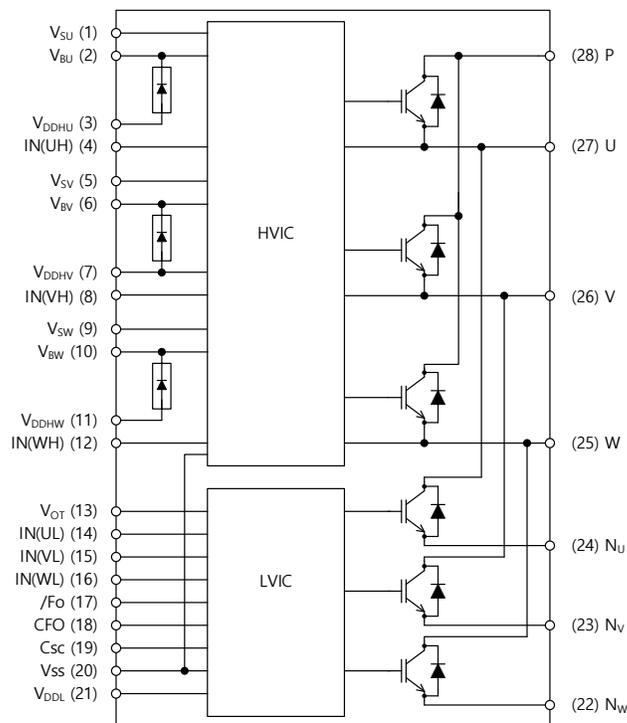
Figure 1. Internal Circuit
